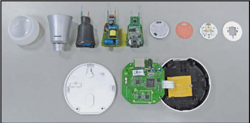
Figure 1. This is what makes hue . In the upper row the various components that make up the bulb; below, the Bridge.
